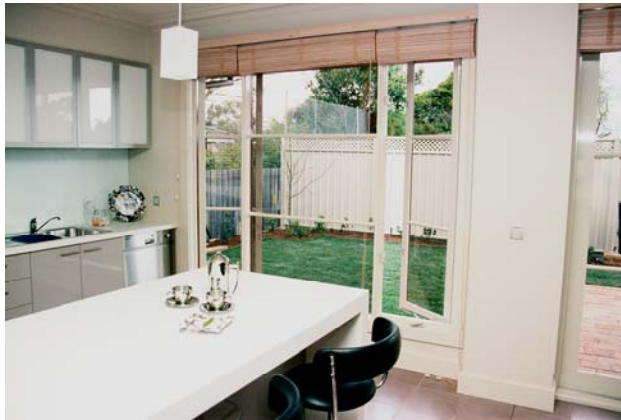
Casement Window - combination casement/fixed lite/casement
